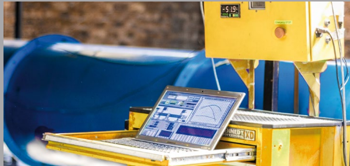
After final assembly, fans are tested according to the ISO 5801 testing standard.
