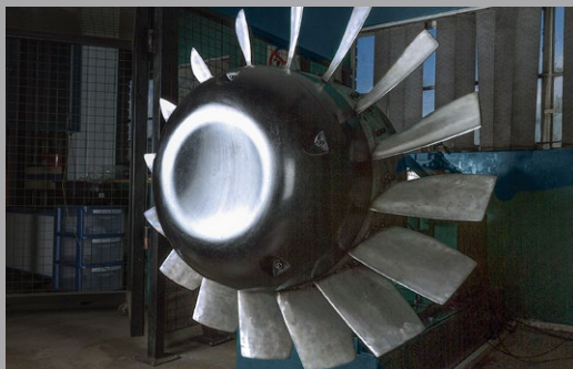
A 1220mm high-pressure variable-pitch impeller on the balancing station
