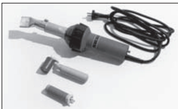
Leister Triac 1460 W hand-held hot air welder, pressure roller and spare element.
