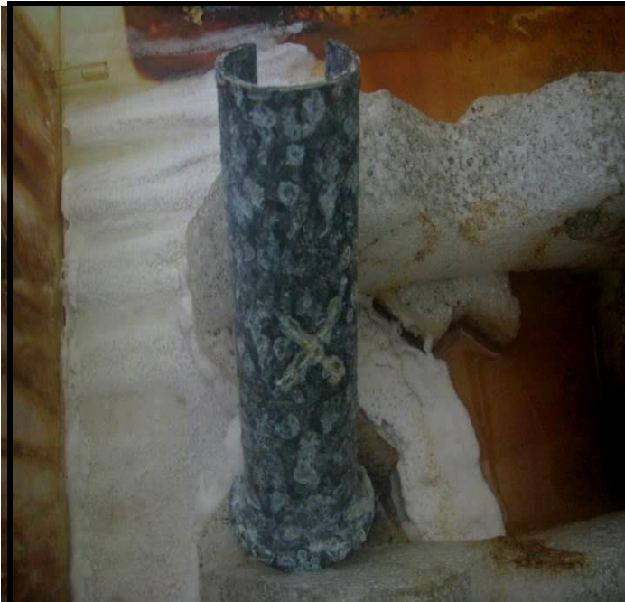
Photograph 29 showing the Sample 1 surface after 168 hours of continuous salt spray exposure.
