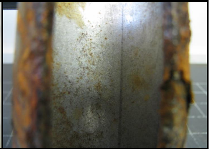
Photograph 18 showing the inner surface of Sample 2 after the 1000 hour exposure.
