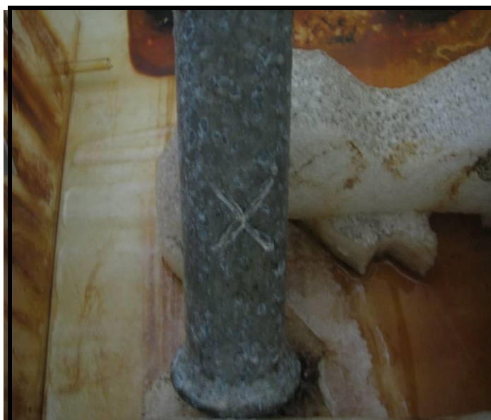
Photograph 23 showing the Sample 1 surface after 24 hours of continuous salt spray exposure.
