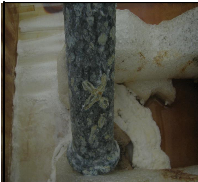
Photograph 31 showing the Sample 1 surface after 336 hours of continuous salt spray exposure.
