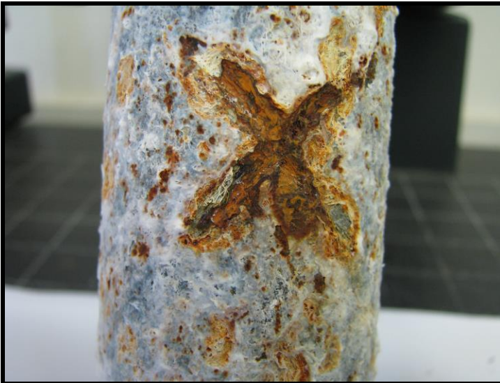
Photograph 11 showing the severe corrosion deposits present in the scribed section of Sample 1 after the 1000 hour exposure.
