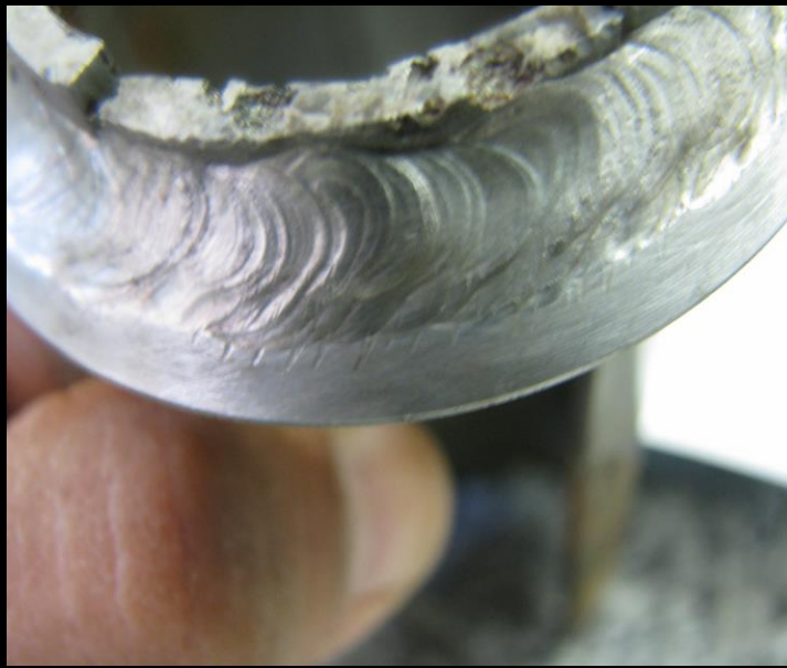
Photograph 19 showing the Sample 2 weld after mechanical and chemical cleansing.
