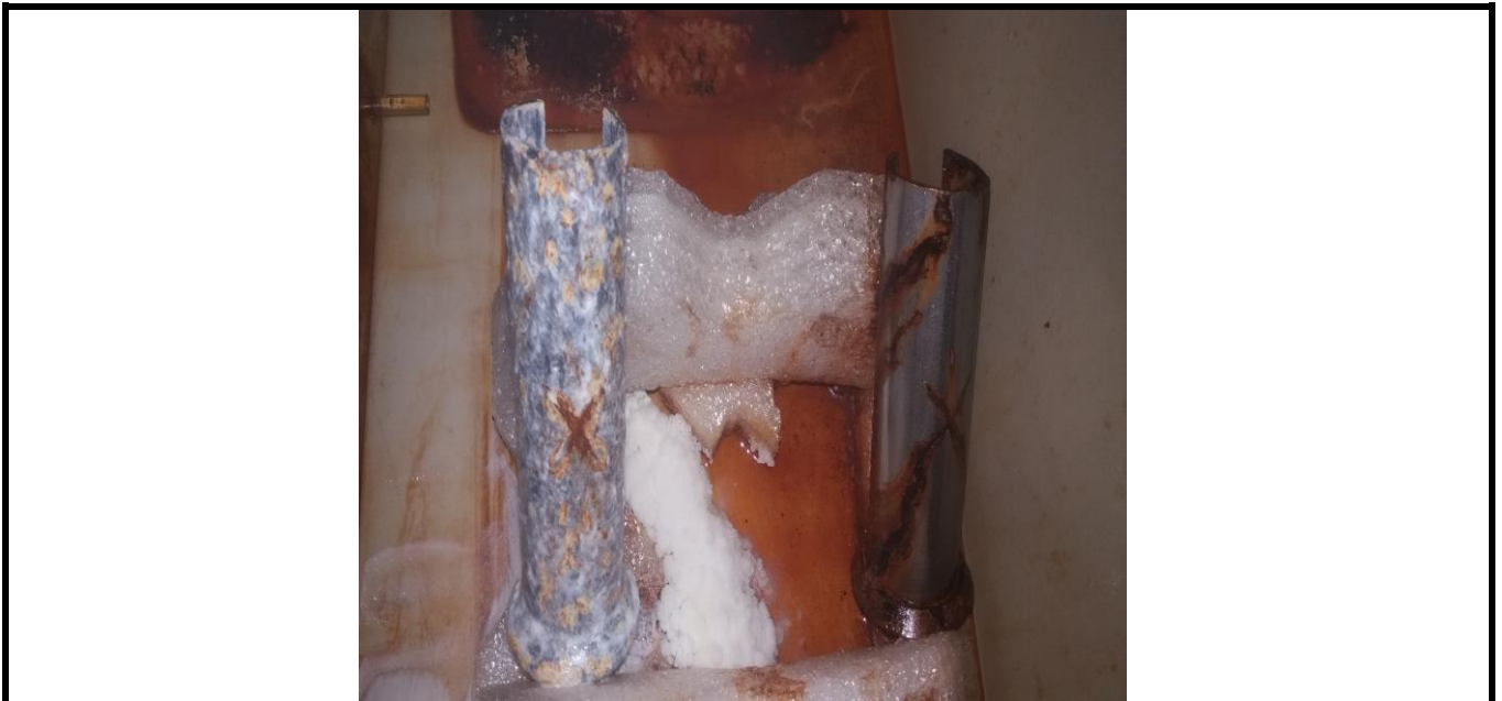
Photograph 37 showing the Sample 1 and Sample 2 surface after 840 hours of continuous salt spray exposure.
