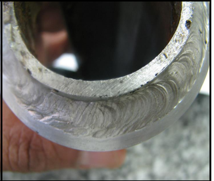
Photograph 20 showing another area of the Sample 2 weld after both mechanical and chemical cleansing.
