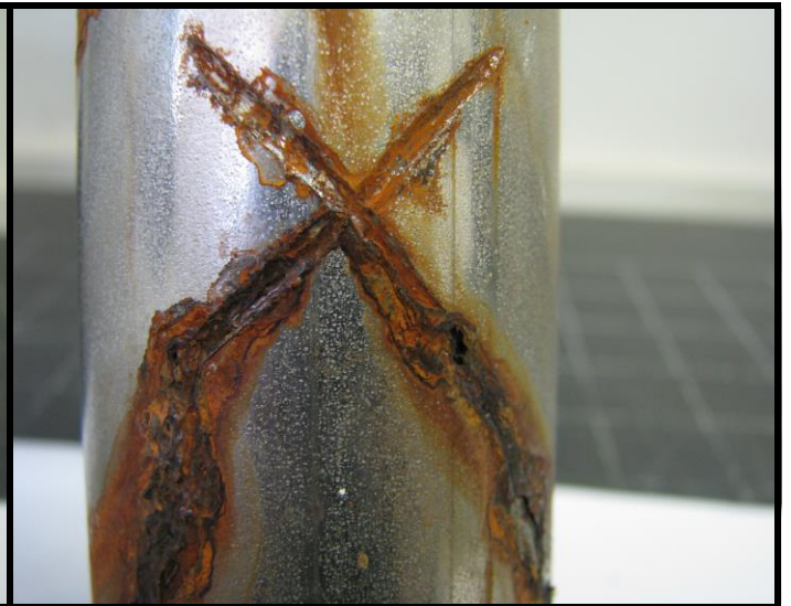
Photograph 12 showing a close-up of the corrosion and run-off staining in the scribed section of Sample 2 after the 1000 hour exposure.
