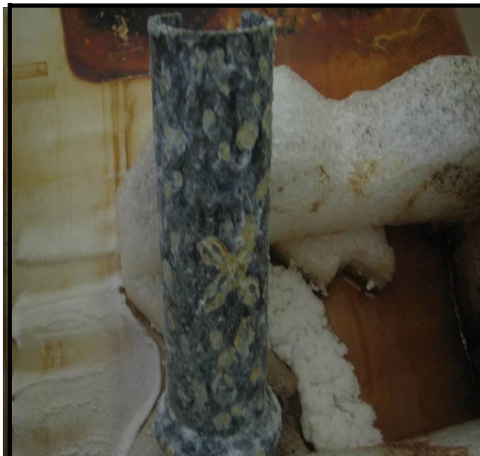
Photograph 33 showing the Sample 1 surface after 504 hours of continuous salt spray exposure.
