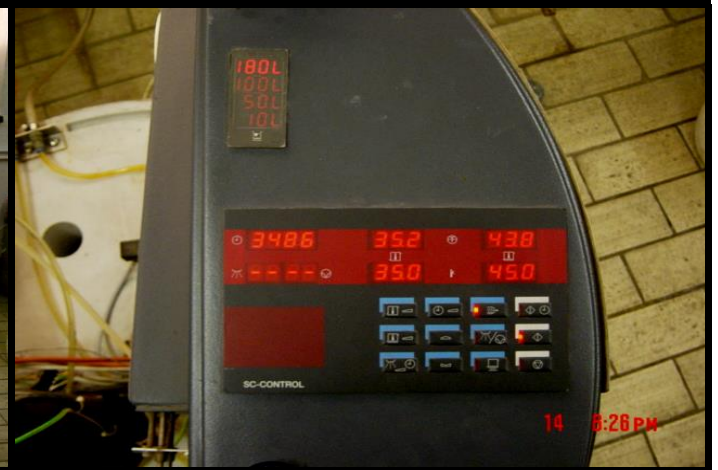
Photograph 2 showing the instrumentation used to control temperature and humidity.
