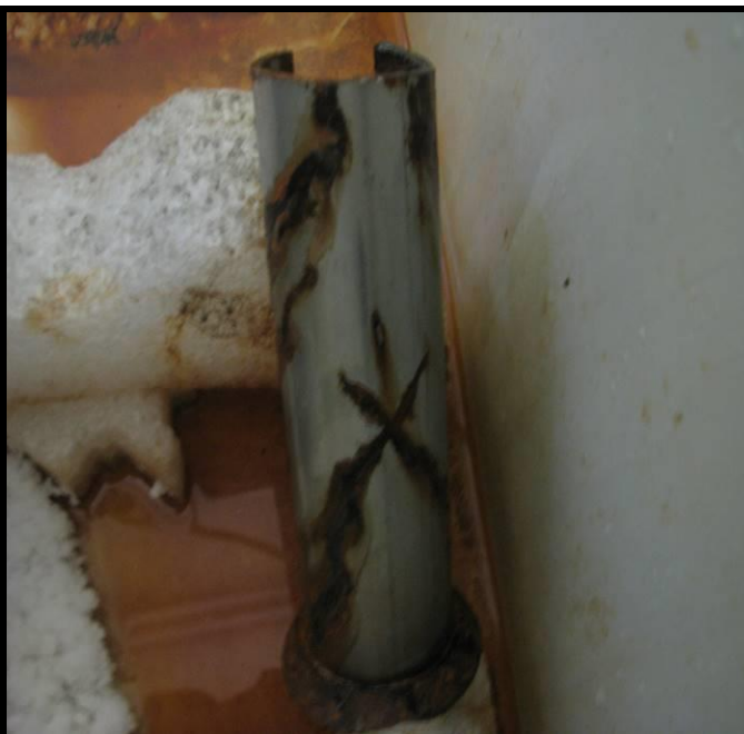
Photograph 34 showing the Sample 2 surface after 504 hours of continuous salt spray exposure.
