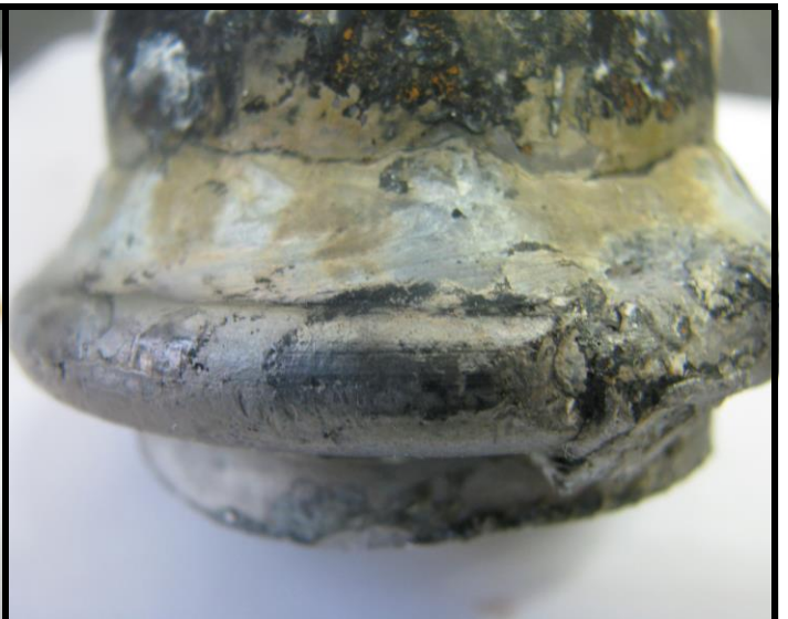
Photograph 22 showing another area of the Sample 1 weld after both mechanical and chemical cleansing.
