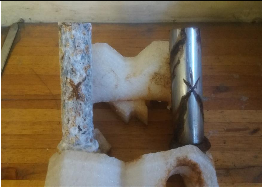
Photograph 38 showing the Sample 1 and Sample 2 surface after the 1008 hours of continuous salt spray exposure.
