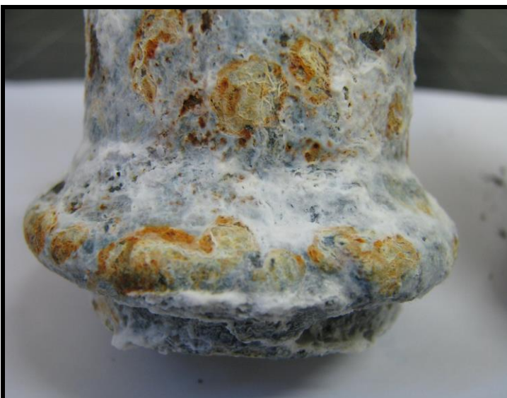
Photograph 15 showing the corrosion on the bottom section of Sample 1 after the 1000 hour exposure.
