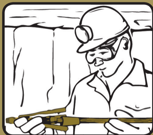
5 Inspect cable bolt for any physical damage. If damaged or missing a component part, do not use.
