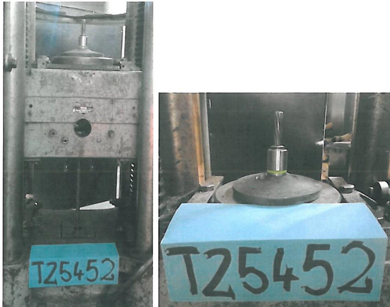
Figure 1. Strands complete with barrel, dome washer and wedge (38 t) installed in the testing machine
