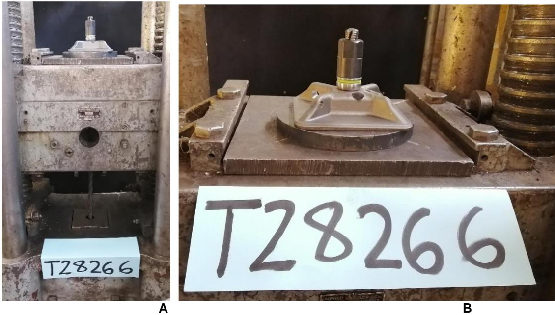
Figure 1. Threaded cable anchor complete with load indicator, nut and 150 mm x 150 mm forged plate installed in the 1 000 kN Amsler Universal testing machine
