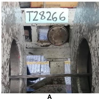
Figure 1. Threaded cable anchor complete with load indicator, nut and 150 mm x 150 mm forged plate installed in the 1 000 kN Amsler Universal testing machine
